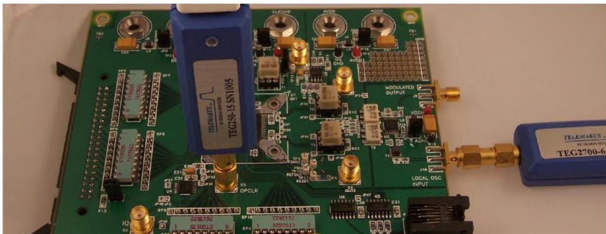
The small size of the TEG devices allow them to be directly connected to the Evaluation board
